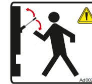
Picture 78: indication of emergency manual pump.
