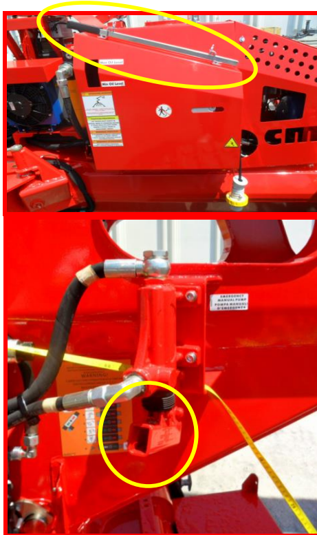
Picture 39: manual pump.
