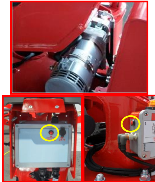
Picture 41: electropump (*optional) activation buttons.
