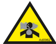
Picture 64: exhaust gas hazard.
