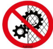
Picture 62: prohibition to remove safety devices.
