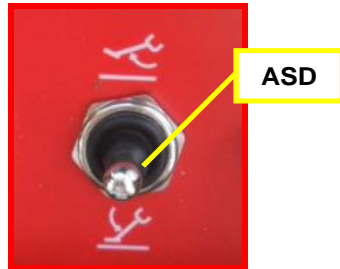
Picture 26: stabilization/destabilization lever on wired remote control.
