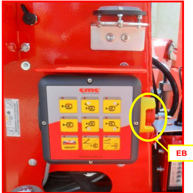
Picture 15: outriggers control station.
